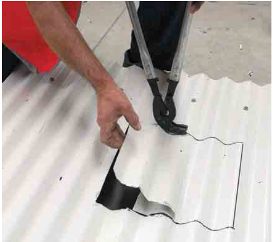
The long arm length of the Metal Pecker allows it to cut through a metal roofing bead or fold cleanly and simply, yet it is small enough to transport easily.
